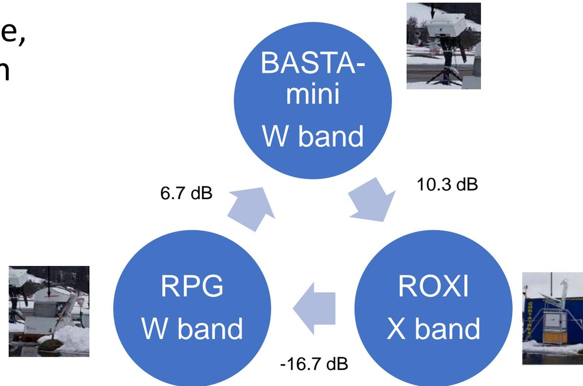
Residual of 0.3 dB after three successive calibration transfers
