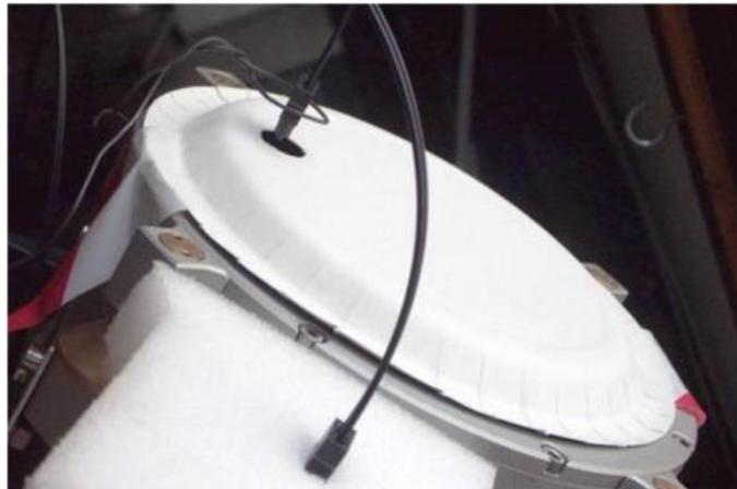
Figure 8: The telescope cover (including the fiber support) (Freudenthaler, V., et al., 2017)
