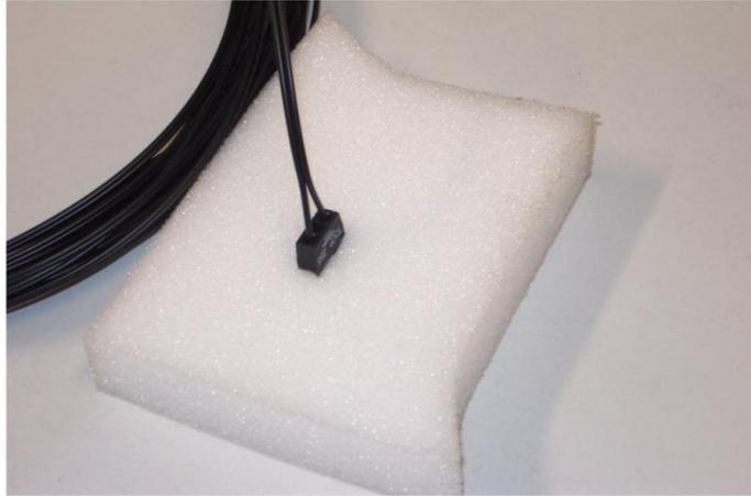
Figure 7: Open-cell foam and communication fiber used for the zero-bin measurement (Freudenthaler, V., et al., 2017).
