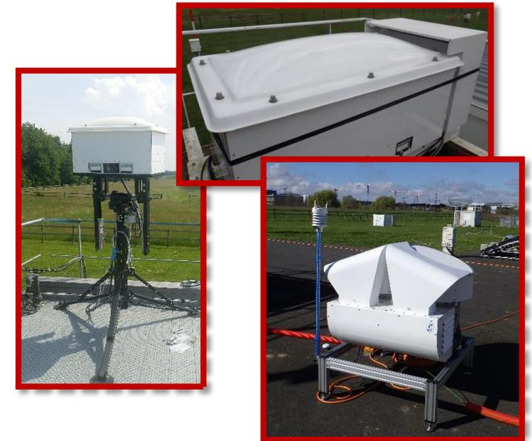
**Doppler Cloud Radar (DCR)** : measure profile of  $Z_e$  (between some tens of meters and several km) with an « a-priori » Calibration Constant that will be checked
