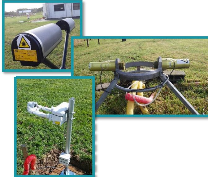
**Disdrometer (DD)** : measure the rain drop size distribution and fall velocity to derive the reflectivity ( $Z_e$ ) at the surface
