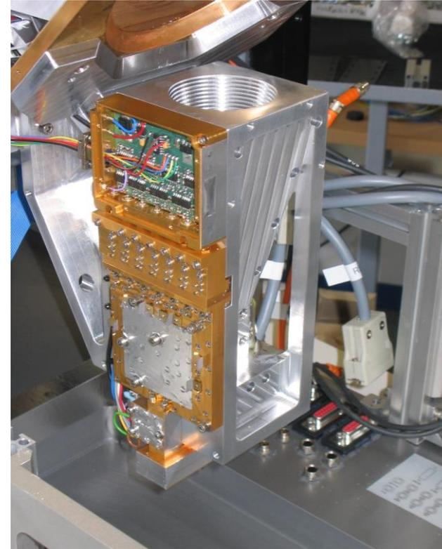
For calibration purposes, a stable noise diode can be switched on to provide a constant additional signal ( $T_N$ )
