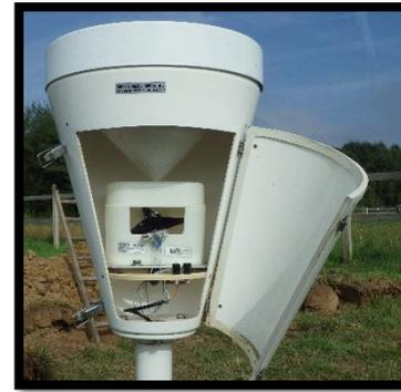
**Rain-Gauge (RG)** : check the DD measurement and detect start/end of the rain event
